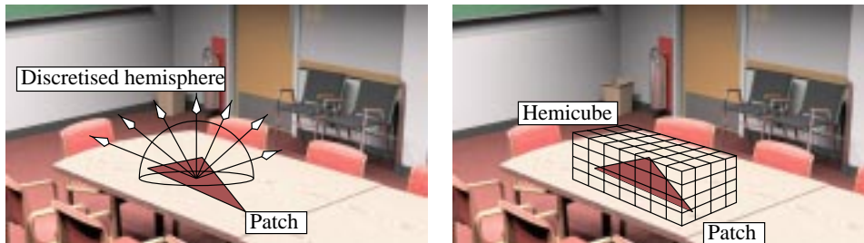
Figure 9: Form factor computation by hemisphere and hemicube methods
