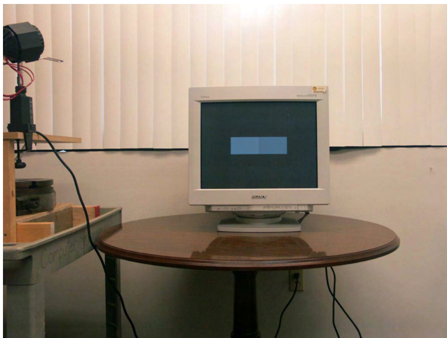
Fig. 7. A photograph of the experimental set-up, taken from the view of the participants. The fluorescent lights of the room were off during the experiment, and the only lighting was provided by the GretagMacbeth D 65 daylight simulator, which illuminated the white surface behind the monitor, as shown.
