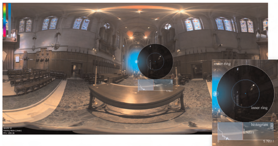
Fig. 1. Quantitative HDR painting interface. In the upper left, a hue and saturation selector is displayed and clearly visible when rendered in color; and in the center and inset, a brush interface is provided that moves with the cursor. In the histogram, the entire luminance domain is visualized and the user selects the luminance associated with the selected hue and saturation values. The highlighted area of the histogram represents the visualized luminance range in which the region within the outer ring is linearly compressed and displayed. The inner ring represents the region that will be painted by the brush. Background image courtesy of Paul Debevec.
