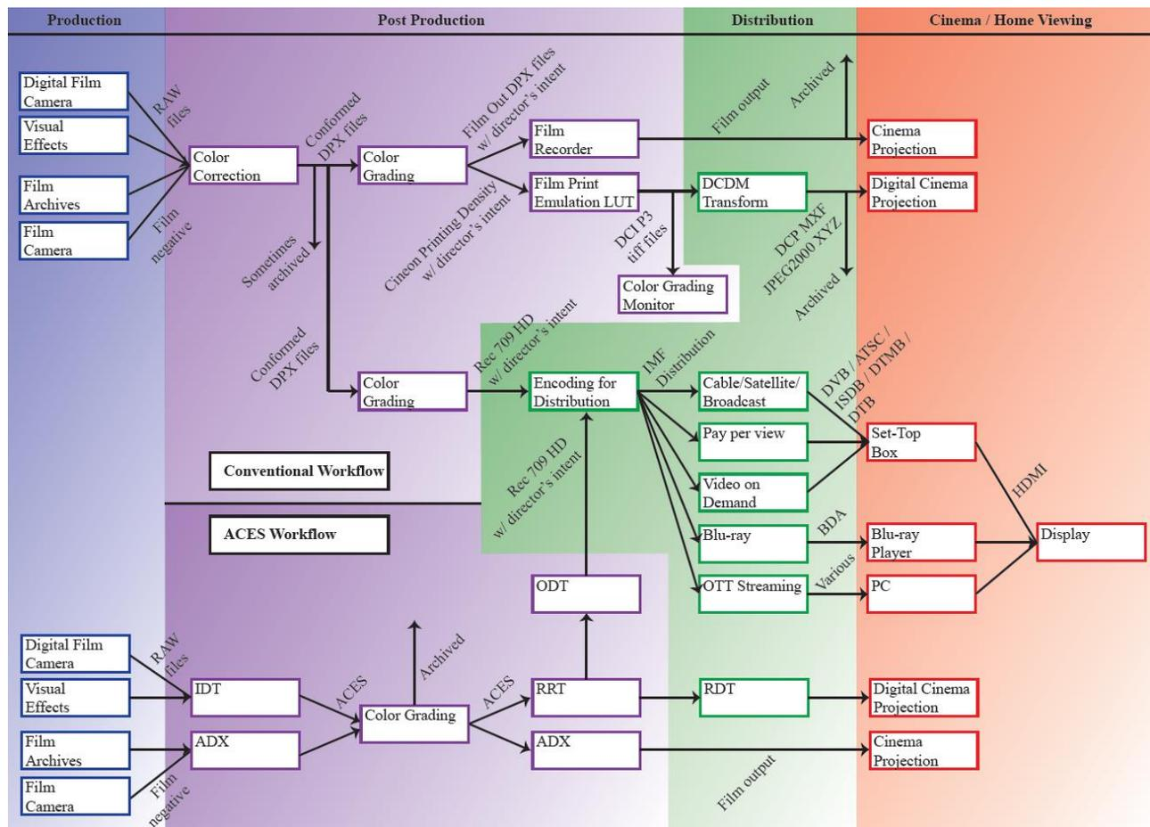
Figure 1. The flow of video data from capture to post-production, distribution, and finally display both in the cinema and at home. Conventional post-production as shown at the top, while the ACES workflow is shown at the bottom.
